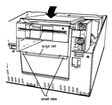
Guide the tabs on the front of the subassembly over the opening in the front of the computer so the two small tabs sit behind the opening and the large tab with the curved lip sits over the front of the opening. If necessary, press on the large tab until the subassembly snaps into place.
